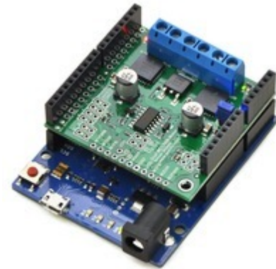
Pololu dual MC33926 motor driver shield, assembled and connected to an Arduino Leonardo.
