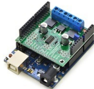
Pololu dual MC33926 motor driver shield, assembled and connected to an Arduino Uno R3.
